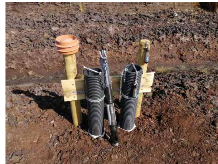
Figure 15. Carbon monitoring project on one of our participant farms allows us to integrate the delivery of carbon, water and biodiversity benefits into the scoring system. The larger probe on the left measures pH and redox every 30 minutes, the small logger measures water table, the logger attached to wooden log on right is atmospheric pressure needed for adjusting and computing water table depths below peat surface. These provide some of the data required to calculate the carbon impacts of the site. Photo courtesy Dr. Amey Tilak.
